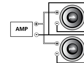
With the coils wired in series and the speakers wired in parallel: 2 dual 4 Ohm speakers will present a 4 Ohm load.
